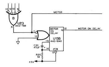
If you look at the schematic of U15B, you can see that C30 gets its power through R20, a 1 Megohm resistor to the +5Vdc power supply. However, you may also note that the capacitor symbol is upside down, the curved part should be negative, flat side to positive, but we are being picky.
