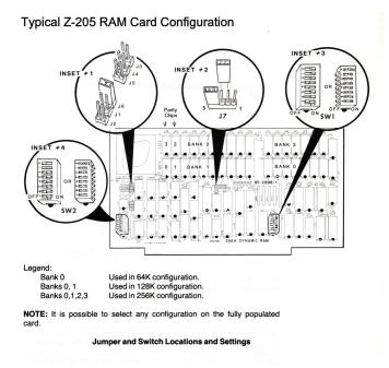
These tests showed that a few bad chips were showing up as alternating values in the data block on display. For example in Bank 1, an alternating 32,33,32,33,32,33... in a block in the display indicates a very bad chip that was causing all the memory reporting problems and boot issues!
