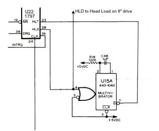
This resistor is in the timing circuit of U15A, a multi-vibrator which provides the Head Load Timing (HLT) signal to U22, the 1797 Floppy Controller, which controls the Head Load signal to the 8" drive connector. When the Head Load Timing signal is low, the drive head is not engaged.
