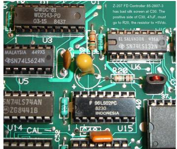
You can clearly see the traces in the closeup. If you compare this with the circuit above, you can see that this is clearly wrong. Also, I checked the card's operation and the motor for the floppy drive never stopped! I reversed the capacitor and now the drive motor lasts about 18 seconds. Please note, and check your 85-2807-3 circuit boards!
