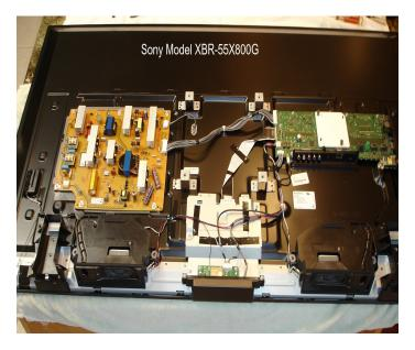
The left yellow board is the power supply, the right long green board is the main board of concern, and the 'T-con' board of many of these models fits between these two boards with the input from the main board via flat ribbon cable and the output via two broad flat ribbon cables going to the screen input below.
