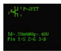
JFETs can have an N-type or P-type channel. In the N-type, if the voltage applied to the gate is less than that applied to the source, the current will be reduced (similarly in the P-type, if the voltage applied to the gate is greater than that applied to the source). A JFET has a large input impedance (sometimes on the order of 1010 ohms), which means that it has a negligible effect on external components or circuits connected to its gate.
