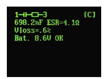
For measuring capacitance, the Tester's capacitance values are computed from the time constant created by the serial connection of built-in resistors and capacitor during charging.
