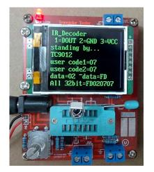
When entering the IR Decoder Function, Row 2 of the LCD shows a string " $\overline{1}$ =DOUT 2=GND 3=VCC". This means to connect TP1 of the tester to the GND of the IR receiver module, and so on. Here are the pinouts for some popular IR Receiver Modules:
