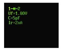
The Tester will cause the LED to flash a few times, then display the diagram of the diode between the two test points chosen, from which you may determine the LED anode and cathode, if necessary. The Uf (forward voltage) value in the range of 1-2Vdc, the capacitance value in the range of 1-30pF and the Reverse Current in nA will be shown.
