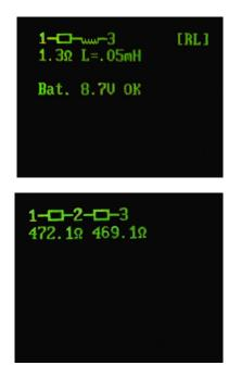
**Note:** If you try to measure small resistor values, you should keep the resistance of plug connectors and cables in mind. The quality and condition of plug connectors are also important. So keep any cable leads short and connectors in good condition.
