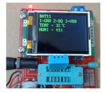
The Tester measures temperatures from 0 to 50 degrees Centigrade and measures relative humidity from 20-90% RH.
