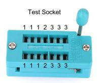
The Test Points in the test socket are arranged in the pattern displayed on the circuit board silk screen just above the test socket. The left six (3+3) belong to TP1, the middle two (1+1) belong to TP2, and the right six (3+3) belong to TP3.
