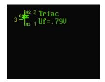
TRIACs are a subset of thyristors and are related to Silicon Controlled Rectifiers (SCRs). TRIACs differ from SCRs in that they allow current flow in both directions, whereas an SCR can only conduct current in a single direction.
