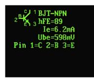
For normal measurement of the three pins of a PNP or NPN transistor, the pins can be connected in any order to the measurement inputs of the Transistor Tester.
