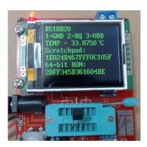
The Tester reads the temperature using 12-bit resolution. It first starts a "Convert T"[44h] command, and then reads a series of 9 bytes of the "SCRATCHPAD" and the "64-BIT LASERED ROM". Fetch the first two bytes within the "SCRATCHPAD" and convert these to the readable temperature shown at row 3 of the LCD.
