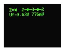
The testing procedure remains the same as a normal diode, which shows a Uf (forward voltage) of about 600-800mV. A zener diode can be detected **if** the reverse breakdown voltage is lower than about 4.5Vdc. It will appear as a double diode, with one direction showing the forward Uf of about 700mV, and the second in the opposite direction with a Uf equal to the **zener voltage** of the diode, in this case, 3.63Vdc.
