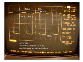
The term duty cycle describes the proportion of 'ON' time to the regular interval or 'period' of time; a low duty cycle corresponds to low power, because the power is OFF for most of the time. Duty cycle is expressed in percent, 100% being fully ON. When a digital signal is ON half of the time and OFF the other half of the time, the digital signal has a duty cycle of 50% and resembles a "square" wave (See the pictures at left and below).
