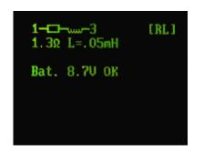
To test, insert an inductor between any two test points.
