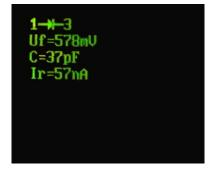
A diagram of the diode between the two test points, the Uf value in mV, the capacitance value in pF and the Reverse Current in nA will be shown.
