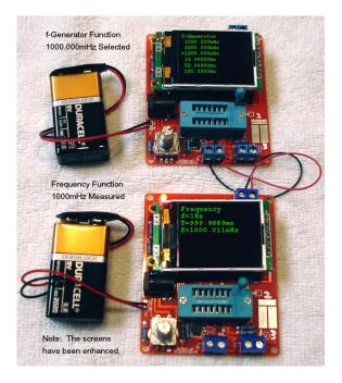
The picture on the left shows two GM328 Testers; the top Tester is generating a frequency of 1000mHz (millihertz or 1Hz) for the bottom Tester to measure. Note the input and output terminals, as these are unmarked on the circuit boards.
