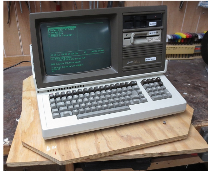
The boards are plywood, about 3/4" thick and 2' x 2' square. The turntable, available from Lowe's, is a 12" size swivel, with a 1000 pound capacity for about $16.00. The screw visible at the right front locks the turntable in position.
