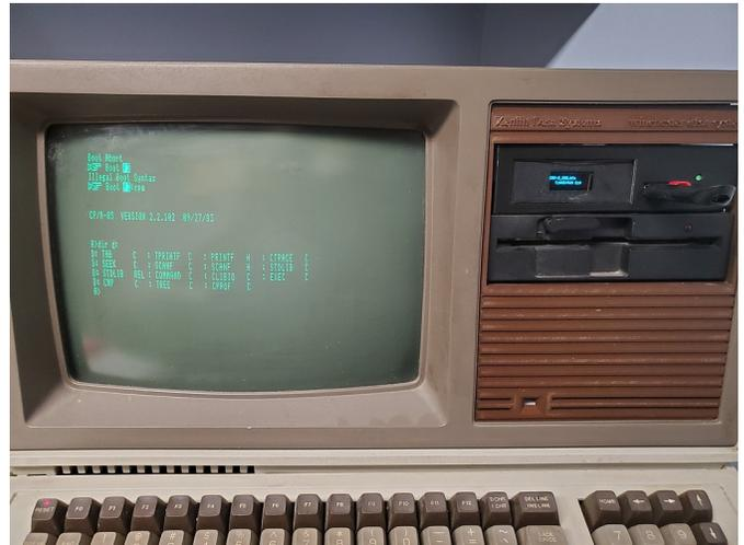
Darrell can easily emulate several different floppy drives by simply selecting the appropriate disk image. It allows him to revive his H-89 and Z-120 by easily transferring applications and data from software repositories or stored floppy disks to a disk image for use in a Flash Floppy Gotek.
