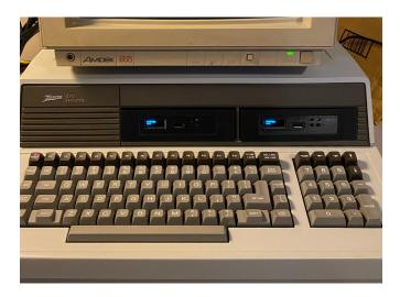
He reports using FlashFloppy firmware from <a href="https://github.com/keirf/FlashFloppy/">https://github.com/keirf/FlashFloppy/</a> - with the OLED displays and a rotary encoder for selecting images (instead of just the buttons). He has been using these on other machines, including an Amiga, Atari ST, and a TRS-80 Model 4P, since floppies are so unreliable these days.
