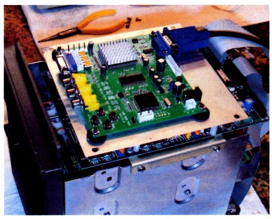
Mount the converter in a manner similar to the first option for the Z-110 - on top of the floppy drive shield, if a dual floppy installation.
