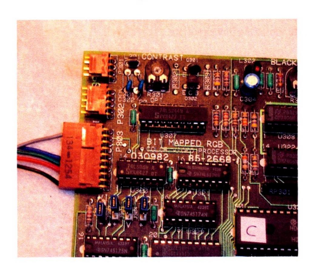
Finally, set the jumpers as shown in the above picture. These are J301 on the left through J304 on the right. From left to right, they should appear to be down, up, up, and up.
