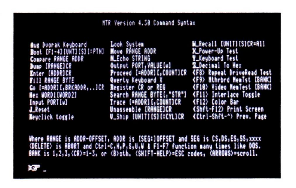
Shown is the MTR ROM version 4.30 boot screen. I suggest you turn on the Z-100 color bar display using the F12 key or the Color Bar menu of the earlier ROMs.
