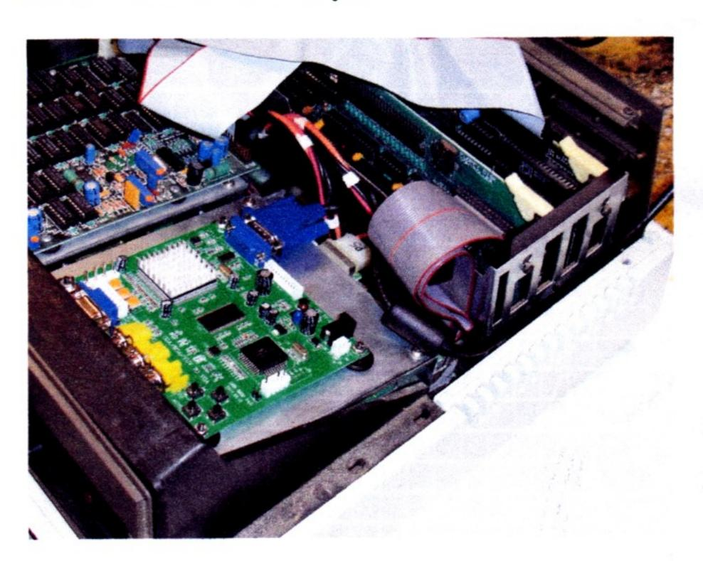
Mounting the converter onto the floppy drive cover is always the easiest. I've used the same approach to adding the 3.5" floppy drive and even adding the IDE Compact Flash card adapters (with modification to the front bezel).
