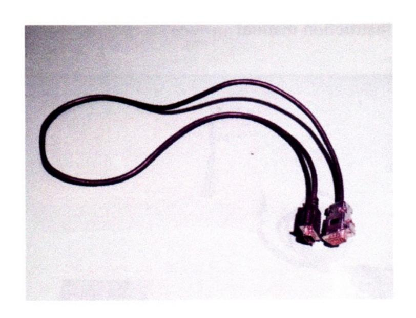
If you don't have good tools and a steady hand, I recommend that you use a commercially made 9-pin to 15-pin cable. What you would need is a male-to-male cable wired pin-for-pin for this application.
