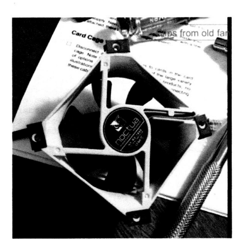
My new fan of choice was a low-noise Noctua NF-R8 fan purchased from Coolerguys.com. The NF-R8 has an acoustical noise value of 17.1 dB(A) and an airflow rating of 53.3 m3/h (31.4 CFM). The airflow is close enough to be compatible and the noise level is 23 dbA less than the stock fan. 17.1 dB(A) is equivalent to a human whisper so this new fan should effectively cut fan noise to zero.
