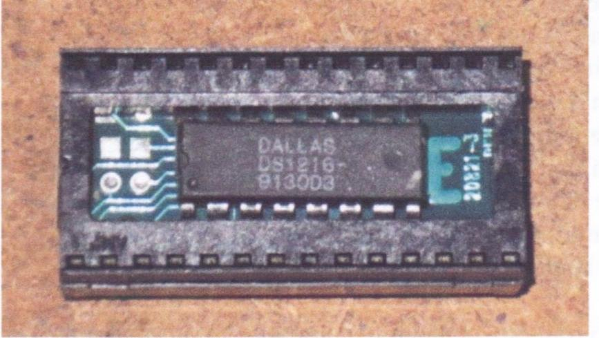
The DS1216E consists of a twenty-eight pin IC socket with a printed circuit board on the bottom that contains a round 3v battery possibly similar to the CR927 which is 0.37" in diameter and a clock controller integrated circuit probably like the DS1315 chip although the chip on the board is marked with the overall assembly part number. The top side of this chip is readily accessible. The bottom where the battery is located is potted with epoxy.
