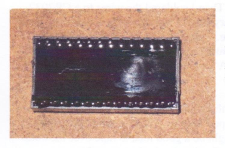
A close examination of the bottom of the DS1216E showed a ghost of the battery and one of its leads. It is difficult to see in this picture but it is there approximately between pins 5 and 23. (Pin 1 is lower right.) I had thought that the battery would be near the other end of the chip but this was not the case.
