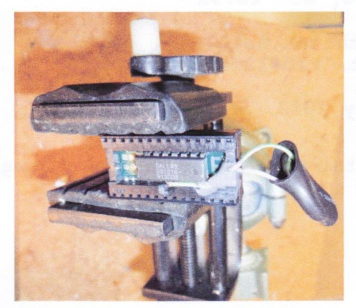
I checked the voltage at controller pin 4 with respect to controller pin 8 and it was +3.2vdc. Pay attention to the polarity here. It could be easy to get it backward. When all was ready, I installed the socket in the Z100 and plugged in the EPROM. Then I accepted a great suggestion from my wife and fastened the battery to the top of an adjacent IC with a couple of small strips of Velcro. For now it seems secure. I don't know what will happen to the self-adhesive of the Velcro over time.
