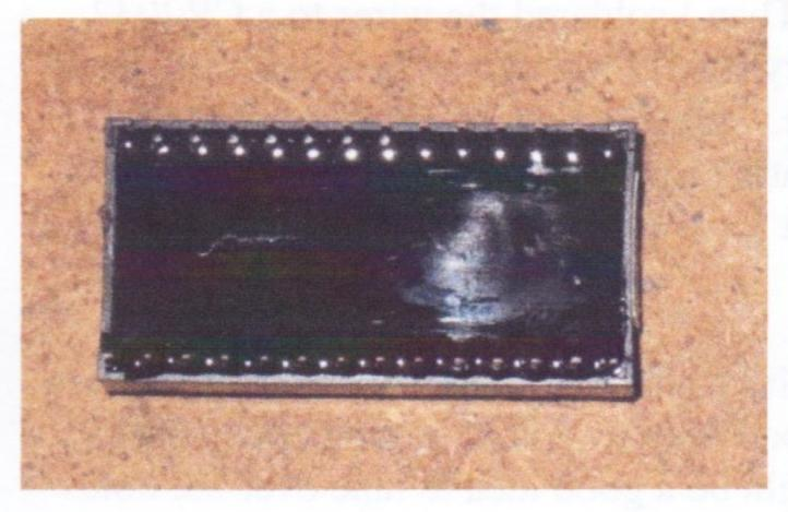
A close examination of the bottom of the DS1216E showed a ghost of the battery and one of its leads. It is difficult to see in this picture but it is there approximately between pins 5 and 23. (Pin 1 is lower right.) I had thought that the battery would be near the other end of the chip but this was not the case.
