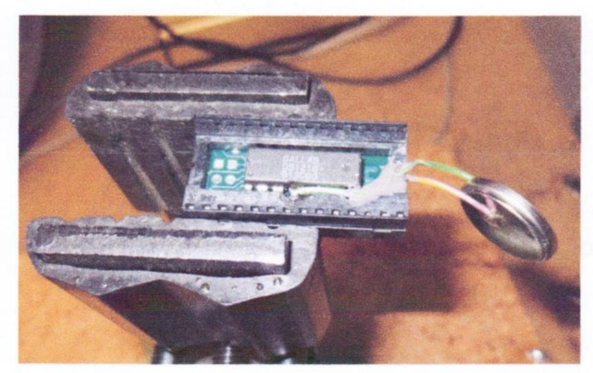
After having everything soldered, I potted the wires in place with JB Weld two part epoxy. Avoid getting epoxy in the socket holes. It might be a good idea to tape over the holes during the potting. Don't ask why I suggest this.
