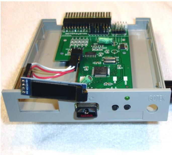
Here is how the OLED looked just before installing in the Gotek.
