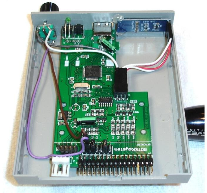
Rotary Encoder and OLED Display Installation
