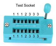
The Transistor Tester has three Test Points (TP1, TP2, TP3) within the test socket and three pads for surface mount components.
