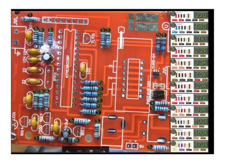
Next, install the resistors. You can install them one at a time, or insert all the resistors, bending the leads slightly to keep them in place, then turning the board over and soldering all the leads at once, clipping off the excess leads as you go.
