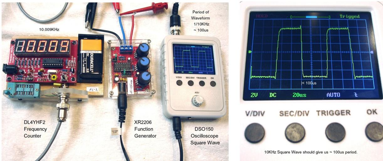
As you can see, I'm using our DL4YHF2 Frequency Counter, our XR2206 Function Generator (set for a 10KHz square wave), and our new DSO150 Oscilloscope to show the waveform.
