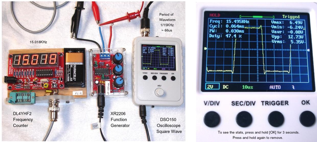
I set the frequency of the square wave to 15.018KHz. If we do our calculations as before, at 15KHz, we should have a period of about 66us. But, this inexpensive oscilloscope can do all the calculations for you automatically. Simply press [OK] to hold the waveform, then press and HOLD the [OK] button for 3 seconds to get this display. Press and hold the [OK] button again to remove the stats from the screen.
