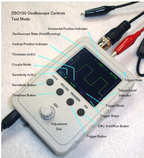
**[V/DIV]:** The [V/DIV] button selects the Sensitivity OR VPOS (Vertical Position Indicator), alternately with each press.
