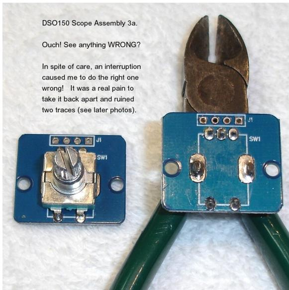
[ ] Mount the Rotary Encoder to the side of the circuit board with the silk screen box. The encoder will snap into the large mounting holes, with the various leads going into their respective small holes.
