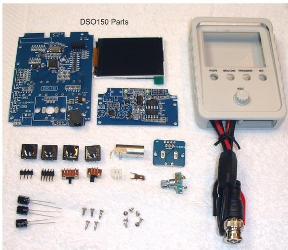
As I already mentioned, with the partly assembled kit, there are only a few remaining parts to install. However, soldering skills are required. If you are new to soldering, I recommend doing some practice before hand. If you do make a mistake and you create a solder bridge, use the solder wick to remove the excess solder (see comments below).
