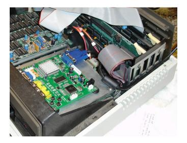
Mounting the converter onto the floppy drive cover is always the easiest. I've used the same approach to adding the 3.5" floppy drive and even adding the IDE Compact Flash card adapters (with modification to the front bezel).
