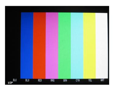
Verify that the proper colors are displayed and in the correct sequence. If the colors are wrong, check and correct the Z-100 to converter cable.
