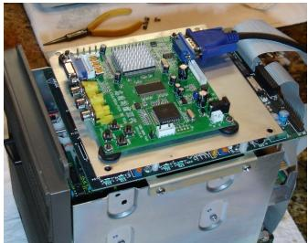
Mount the converter in a manner similar to the first option for the Z-110 - on top of the floppy drive shield, if a dual floppy installation.
