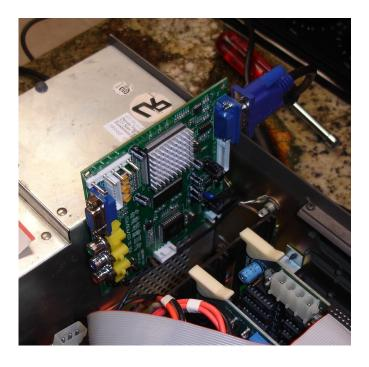
This one is more difficult and isn't for the faint hearted. If you look beside the right side of the power supply of the low profile computer, you will find what appears to be just enough space to mount the converter on the right rear corner of the power supply, though obviously not in this position. This picture was just meant to show the relative sizes. You would need to lower the converter so the top edge is about level with the top of the power supply.
