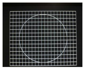
I found when setting the vertical size, I would see undesired lines at the bottom of the screen if I went too small. The value given earlier works for me.
